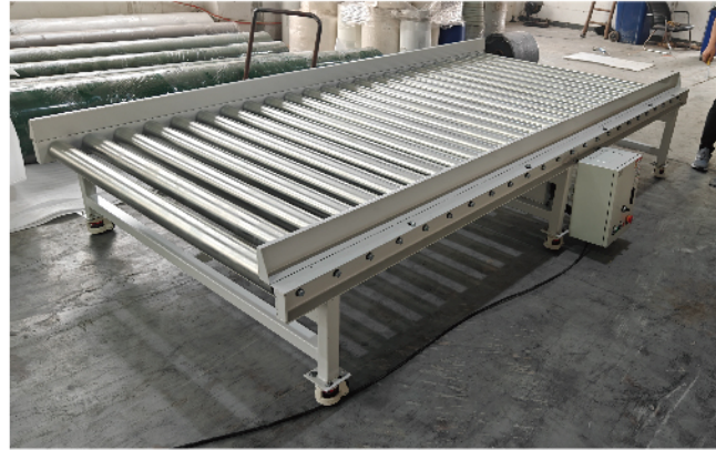
滚筒输送机/Roller conveyor
