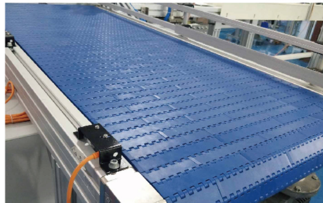
链板输送机/Chain plate conveyor
