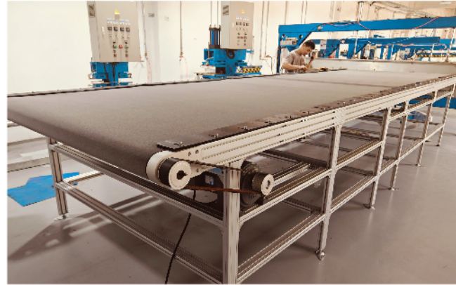
皮带输送机/Belt conveyor
